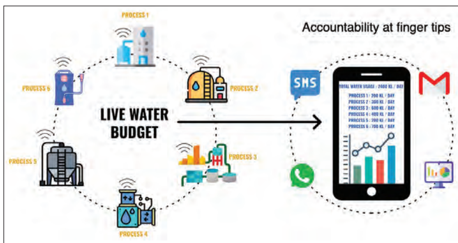
Ultrasonic flowmeters and level meters to track water distribution continuously and transmit the data online
