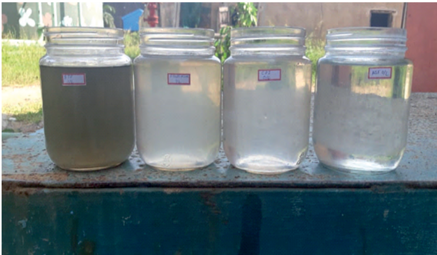
Figure 3: Raw and treated water at different stages (Left to right Surge Tank Inlet, Surge Tank Outlet, CPI Outlet, NSF Outlet)
