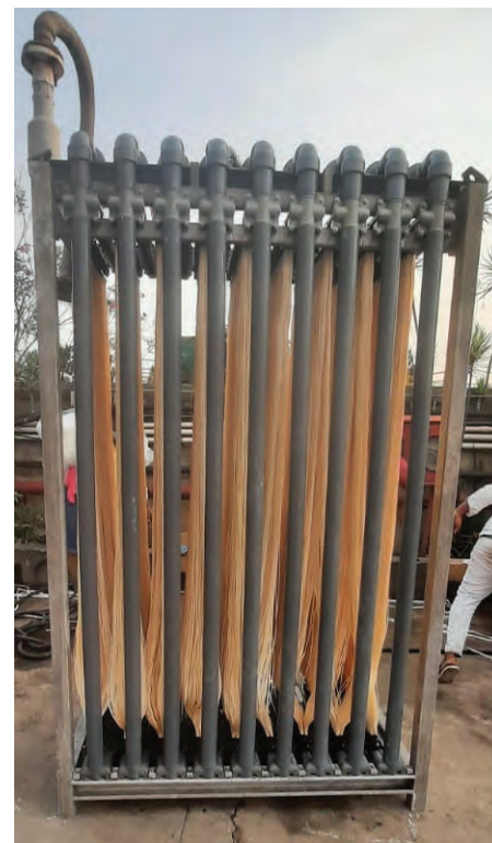
Figure 3: MOWS Ultra–PUREIT Hollowfibre modules ready for installation for food industry, Tamilnadu 2021
